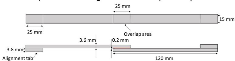
Figure 1 – Single lap joint geometry.
