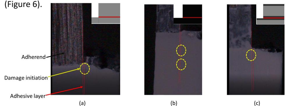
Figure 5 – Damage initiation for (a) conventional composite, (b) thin-ply and (c) hybrid (25% thin-ply) joint.
