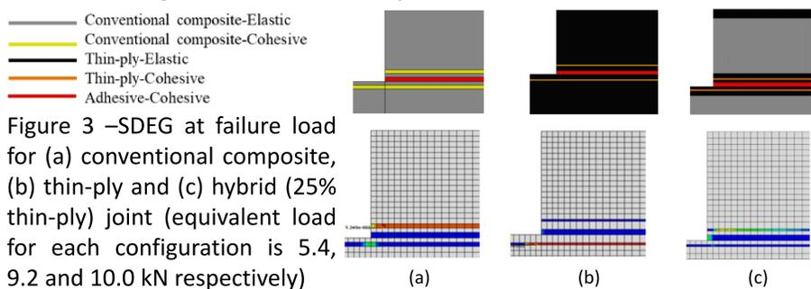
Figure 3 –SDEG at failure load for (a) conventional composite, (b) thin-ply and (c) hybrid (25% thin-ply) joint (equivalent load for each configuration is 5.4, 9.2 and 10.0 kN respectively)
