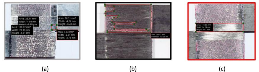
Figure 6 – Representative images of the failure surface of (a) reference conventional composite, (b) thin-ply, and (c) hybrid (25% thin-ply) joint.
