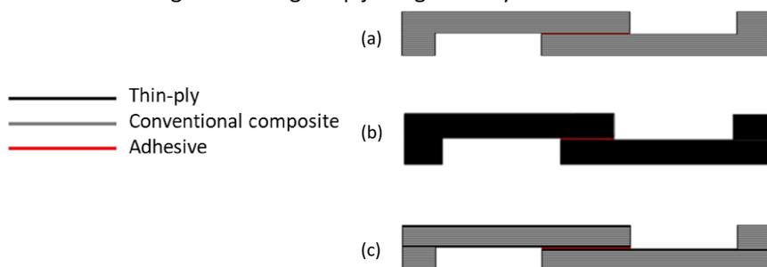
Figure 2 – Schematic design of (a) conventional composite, (b) thin-ply, and (c) hybrid joint (25% thin-ply) joint.
